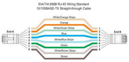
Figure B-2 Straight-through Wiring
